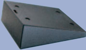
The VCW 15 wedge facilitates the stacking of mid-hi cabinets to suit different requirements concerning radiation angle and aiming. The VCW 15 can be used in both ways creating a vertical angle of 15° up or downwards.
